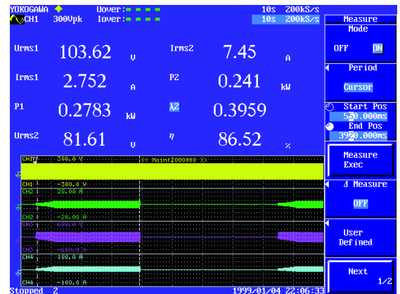
Example of efficiency evaluation when inverter output is turned on in a cooking machine using induction heating
