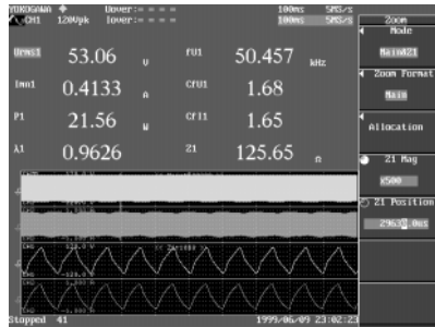
Example of measurements on inverter lighting equipment with a fundamental wave of approximately 50 kHz
